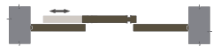
3 ante parallele scorrevoli a soffitto, binario 2 vie Triple parallel sliding door, 2 ways ceiling-rail
