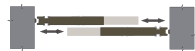
2 ante parallele scorrevoli a soffitto, binario 2 vie Double parallel sliding door, 2 ways ceiling-rail
